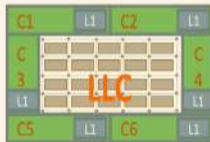
A Chipmultiprocessor (CMP) with non-tiled architecture.
